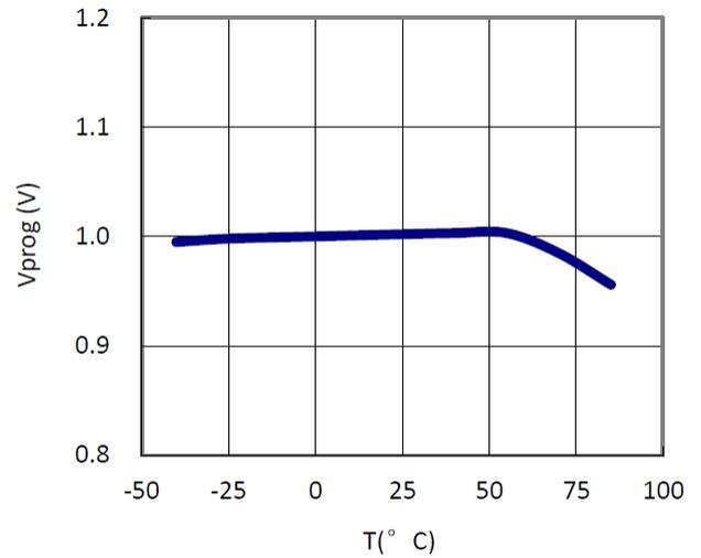
**Recharge Voltage vs Temperature**
