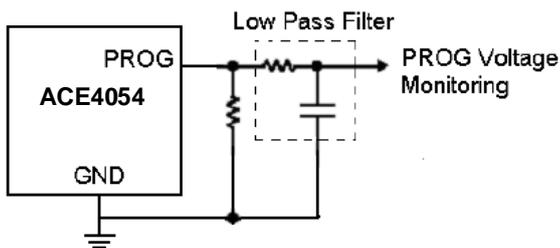
Figure 2. Isolating Capacitive Load PROG Pin and Filtering
