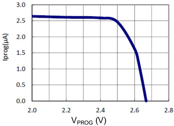
PROG Pin Current vs PROG Pin Voltage
