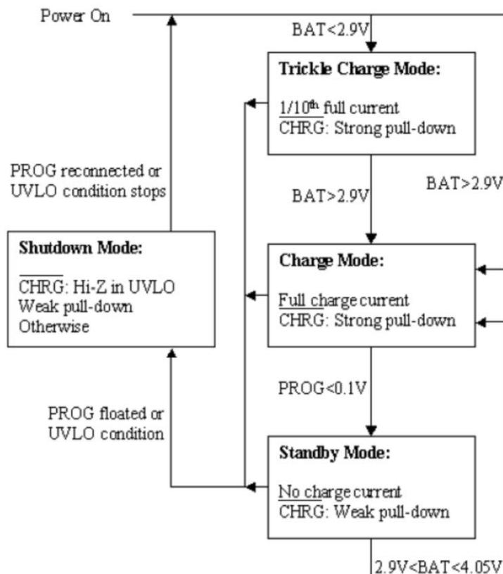
Figure 1. Charge Cycle Diagram
