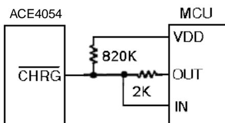
Figure 4. Using a Microprocessor to Determine  $\overline{\text{CHRG}}$  State.
